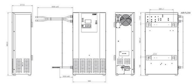
DIMENTIONS (LxWxH): 348x665,50x217,5 mm - 13.70x26.20x8.56 in. WEIGHT: 35 Kg - 77.16 lbs PROTECTION GRADE IP20 INPUT VOLTAGE: 200/208-240/400/440/480 Vac - 50-60 Hz
